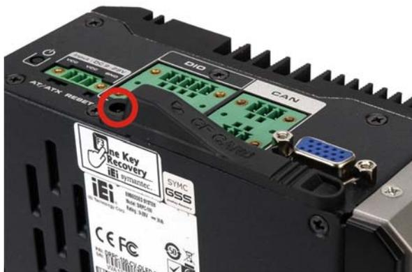
**Figure 3-3: Replacing the CF Card Slot Cover**
