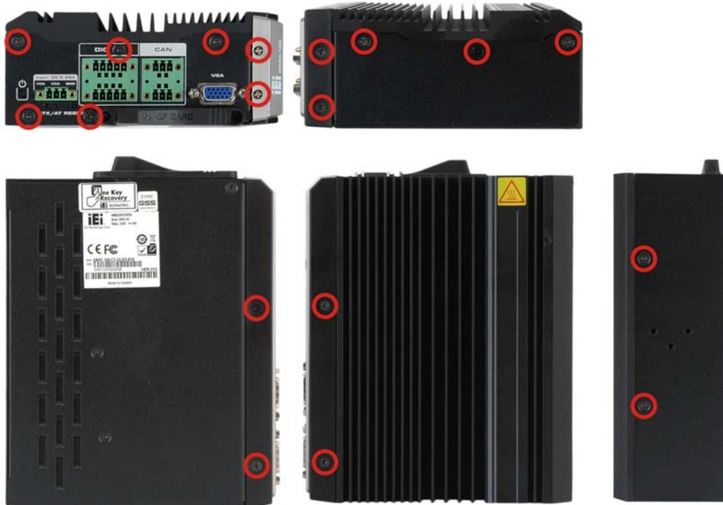
**Figure 3-4: Retention Screws**
