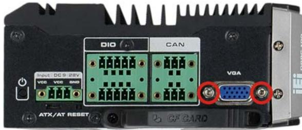
**Figure 3-6: Hex Nuts on the Top Panel**
