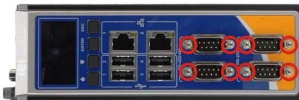
**Figure 3-5: Hex Nuts on the Front Panel**
