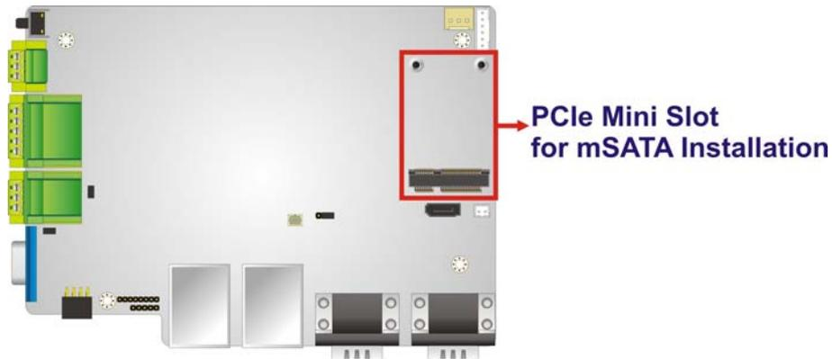
Figure 3-8: PCIe Mini Slot Location
