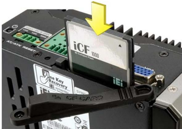
**Figure 3-2: CF Card Installation**
